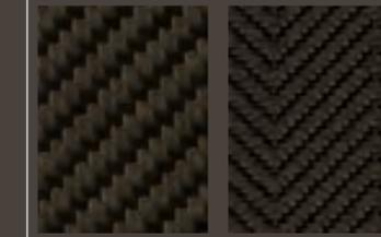
Twill carbon fibre Herringbone carbon fibre
